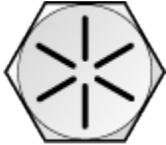
Grade 8 bolts have been hardened more than grade 5 bolts. Thus they are stronger and are used in demanding applications such as automotive suspensions. Grade 8 bolts have 6 evenly spaced radial lines on the head.
