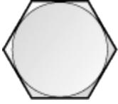
Grade 2 is a standard hardware grade steel. This is the most common grade of steel fastener and is the least expensive. Except a possible manufacturer's mark, Grade 2 bolts have no head marking.
