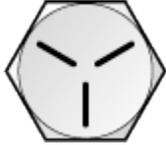
Grade 5 bolts are hardened to increase strength and are the most common bolts found in automotive applications. Grade 5 bolts have 3 evenly spaced radial lines on the head.
